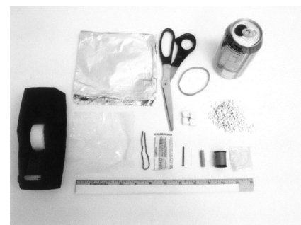
Figure 1. Typical household materials used for the construction of the KFM unit. From the bottom left: tape, ruler, transparent plastic sheet, charging wire, bandage, nail, needle, broken pencil, insulating thread (polyester sewing thread and non-waxed dental floss), standard aluminum foil, scissors, drying agent (drywall and calcium sulfate), and a typical metal can (glue is not pictured).
